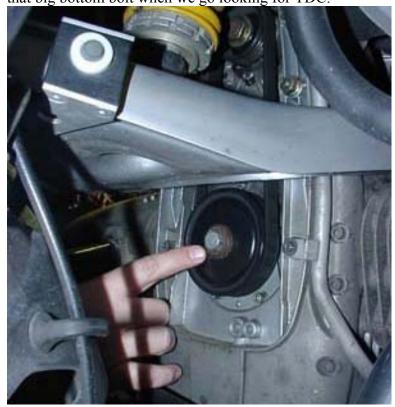
9. You'll find the engine timing on the 'Throttle grip' side of the engine. It's that little round slightly concave rubber plug behind the cylinder head, right up above the throttle body, just below the telelever hinge. Oh, for chrissakes, it's right HERE...
