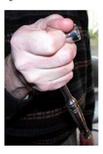
Not only is that too much, you can't use a ratchet because you need to keep the hex wrench locked while torqueing the locknut.
