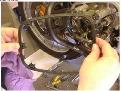
85. Put the rubber spark plug gasket back into/onto the cylinder head cover. You remembered to rotate this gasket so the plug arcs get virgin gasket, right? Ahhhh.
