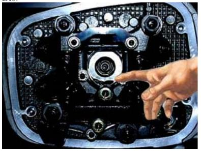
d. Good. First clean the mating area on the cylinder head cover then put the gasket back into place on the cover and rotate the rubber plug gasket about 90 degrees so those it will press virgin flesh against the plug tunnel wall. Ahhhh.
